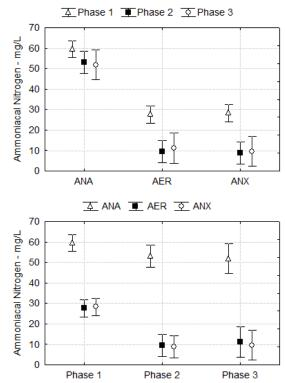
Figure 2. ANOVA factor analysis comparing Ammonia Nitrogen in sampling points and research phases
