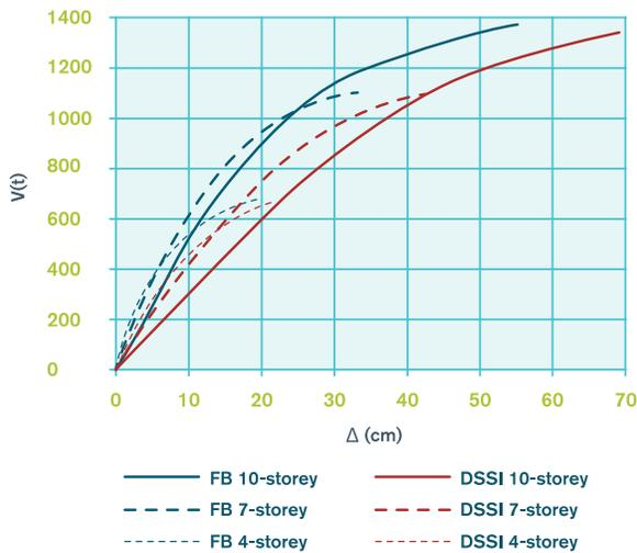
Figure 6: Capacity curves for steel buildings with braced frames with different heights (4, 7 and 10 storeys).
