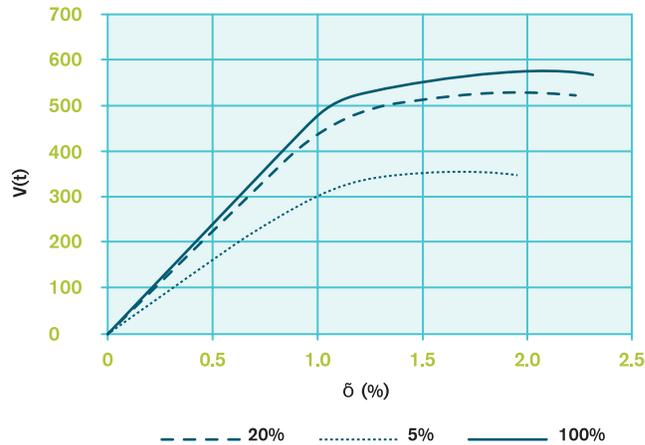
Figure 4: capacity curves with structural deformation ( $u$ ) for unbraced frames with 100%, 20% and 5% soil foundation stiffness.
