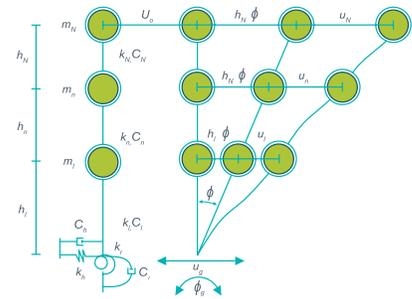
Figure 1: Displacement elements of a structure with a flexible base.
