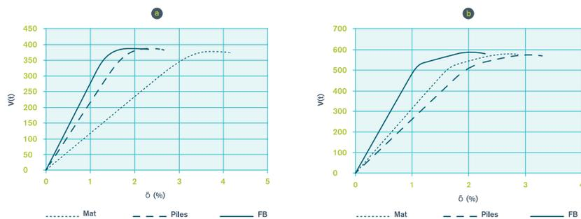
Figure 2: capacity curves with total displacement ( $u$ ) for unbraced frames on a fixed base (FB), mat foundation (Mat) and pile foundation (Piles) for a) 8-storey and b) 16-storey buildings.
