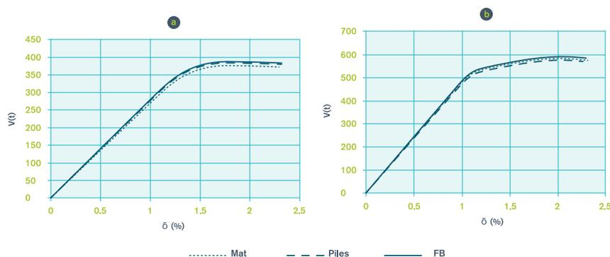
Figure 3: capacity curves with structural deformation ( $u$ ) for unbraced frames on a fixed base (FB), mat foundation (Mat) and pile foundation (Piles) of a) 8 storey and b) 16 storey buildings.
