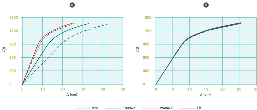
Figure 5: capacity curves for RC buildings on different soil types ( $V_s=70, 100$  and  $250$  m/s) and a fixed base with a) structural deformation ( $u$ ) and b) total displacement ( $\tilde{u}$ ) (figures 5).
