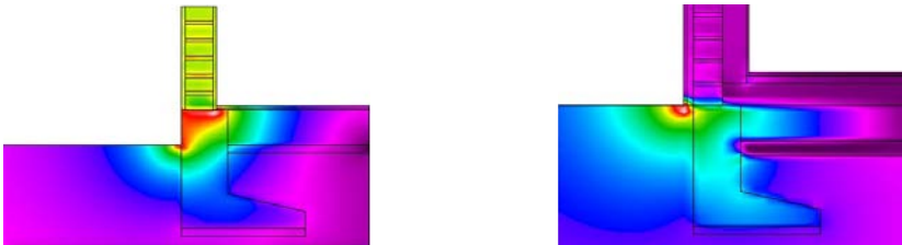
Figure 11: Heat flow through materials in traditional and improved wall / foundation building junction
