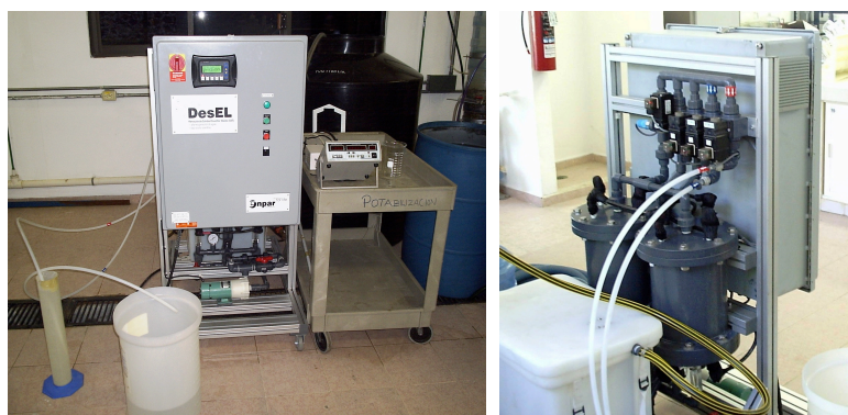
Figure 2. Front view (left) and rear view (right) of DesEL-4k plant showing pure and reject water outlets, deionization cells, and solenoid valves.
