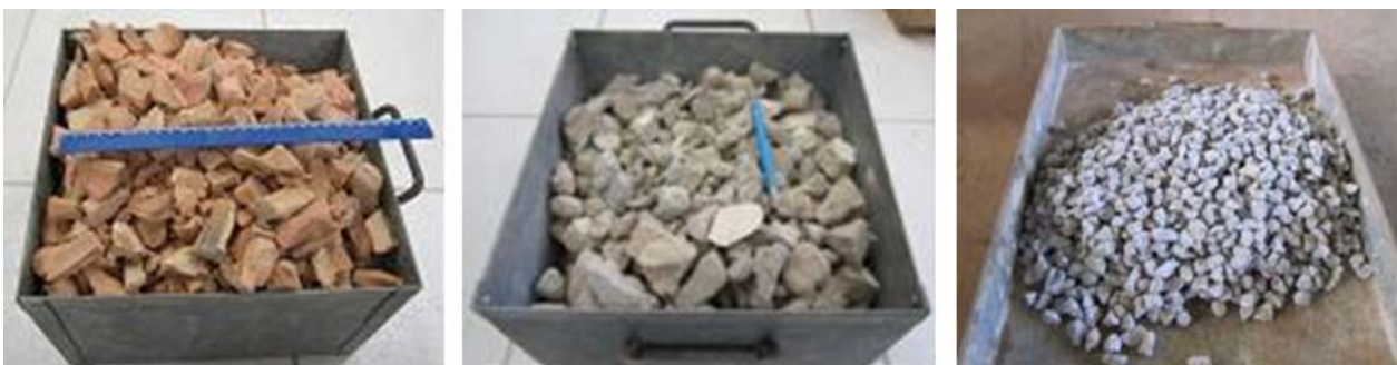
Figure 3. Recycled aggregate: ceramic CDW (left), plaster CDW(center), and concrete CDW (right).
