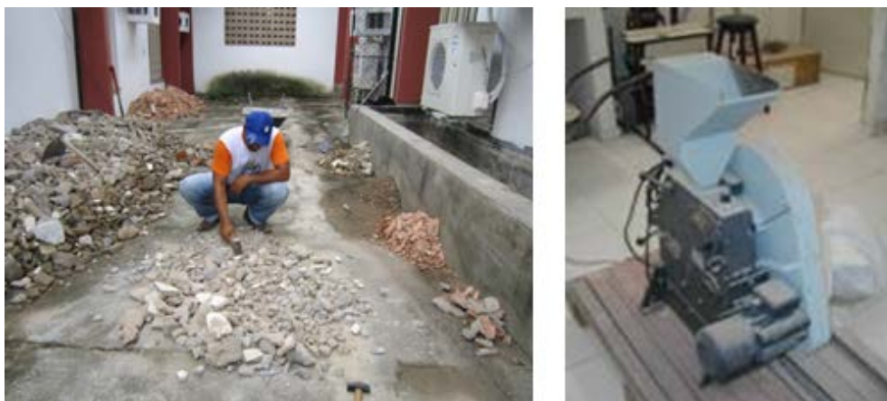
Figure 6. Crushing process: hand-driven crushing (left) and mechanic crusher (right).
