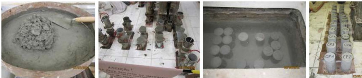
Figure 8. Preparation of the specimen (from left to right): fresh concrete, molding, curing, and striking.
