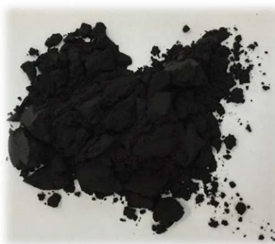
**Figure 5.** RHA obtained by combustion in a grated furnace
