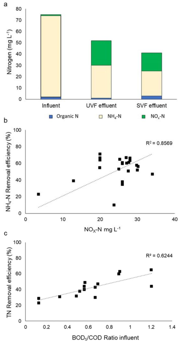
**Figure 2.** Nitrogen transformations in the unsaturated (UVF) and partially saturated vertical (SVF) subsurface flow wetlands. a) Nitrogen species concentrations in influent wastewater, and effluent of the UVF and SVF wetlands; b) Correlation plot of NH<sub>4</sub>-N removal efficiency vs. effluent NO<sub>x</sub>-N in the UVF wetland; c) Correlation plot of TN removal efficiency vs. influent BOD<sub>5</sub>/COD ratio in the SVF wetland.
