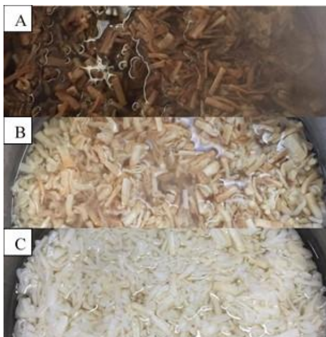
Figure 1. Steps in the process of cooking cigarette butts. a) First step of cooking; b) second stage of cooking; c) rest in sodium hypochlorite solution.
