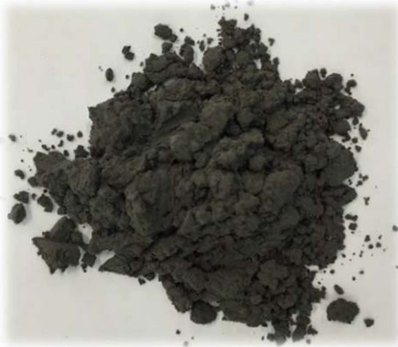
Figure 4. RHA obtained by combustion in a bubbling fluidized bed reactor
