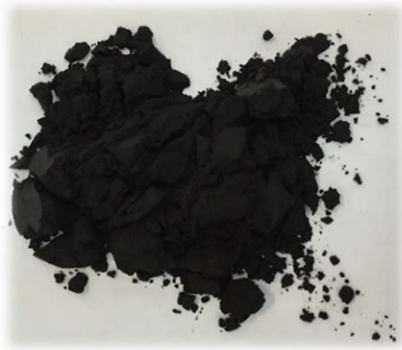
Figure 5. RHA obtained by combustion in a grated furnace
