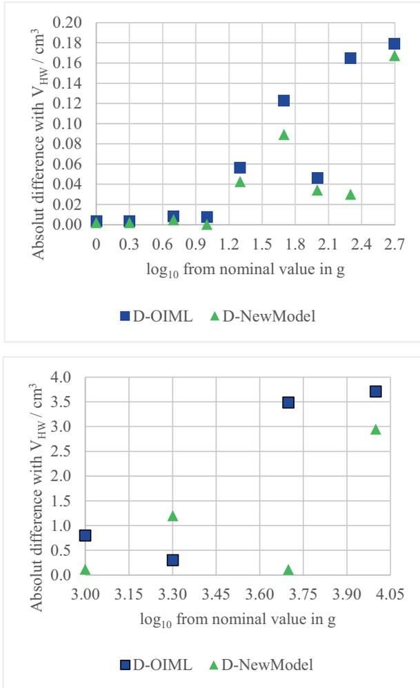
$D-OIML = ABS(V_{OIML} - V_{HW}); D-NewModel = ABS(V_{NewModel} - V_{HW})$ .
