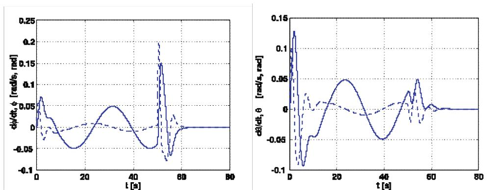
Figure 6. Roll angle  $\phi$  (continuous line) and roll angular velocity  $\dot{\phi}$  (dashed line) (left). Pitch angle  $\theta$  (continuous line) and pitch angular velocity  $\dot{\theta}$  (dashed line) (right)
