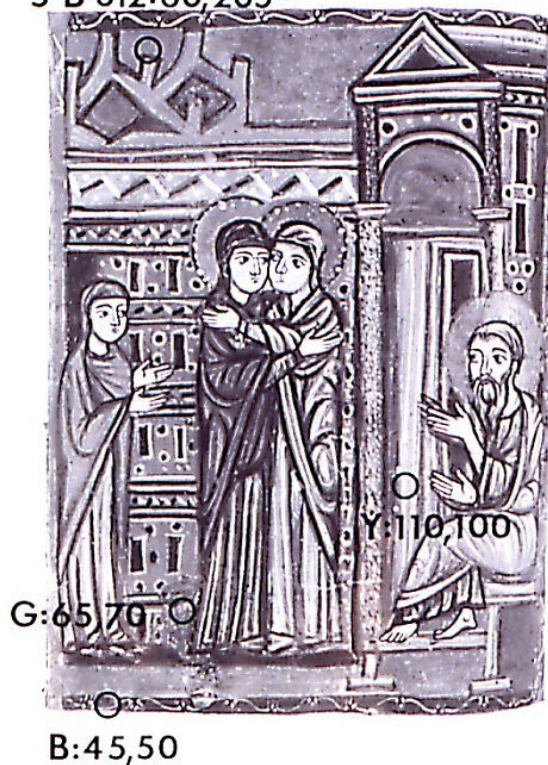
Figure 8. Documentation of an Armenian Manuscript Page Selected for Analysis: The Visitation of Mary to Elizabeth, p. 312 of the Glajor Gospel Book of UCLA (early 14 th century). The circles indicate locations from which samples were taken for analysis. B , Y , and G indicate the hues: blue, yellow, and green; the other numbers are x-y coordinates in millimeters measured from the bottom left corner of the page. Photograph: M.V. Orna
