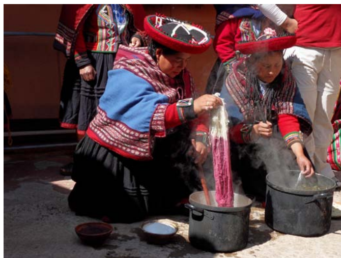
Figure 5. Chinchero, Perú. A demonstration of dyeing of wool fibers with cochineal at varying pH of the dyebaths. Photograph: M.V. Orna.
