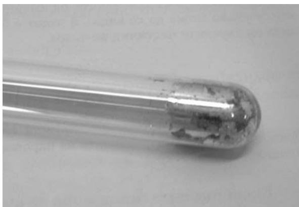
Figure 2. K-Na alloy covers the test-tube glass due to strong adhesion forces
