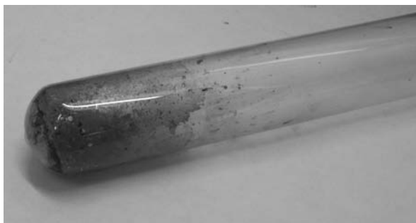
Figure 4. K–Na amalgam is occasionally stuck on the test-tube walls.
