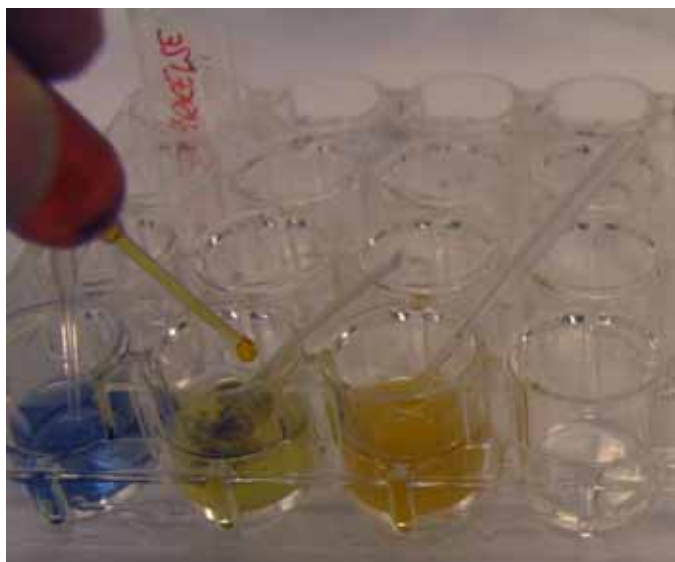
Figure 2. This second figure shows three stages of the titration, the left well is a titrated sample, in the middle a sample during titration and the right one is an untitrated sample.
