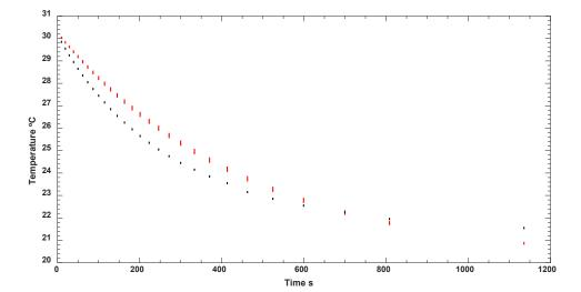
Figure 3. Model-I: (up) 3a – Script 1. (down) 3b - Adjusted temperature with model-I, compared with experimental data |: Red interval-bar of adjusted data and |: Black interval-bar of experimental
