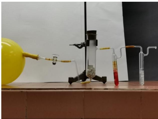
As the wood burns, the stream of oxygen together with the other gaseous products passes through the wash-bottles. Dramatic changes are seen immediately: the light orange color of the methyl orange changed into intense red one, while the clear and transparent solution of lime-water turned foggy (Figure 4). Upon longer bubbling the liquid may or may not turn clear again, as will be discussed in what follows.
