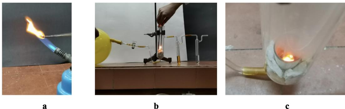
**FIGURE 4.** Bubbling of the excess oxygen with the gaseous products through the wash-bottles induces noticeable changes of the optical properties of the solutions.
