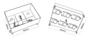
*Note.* The left panel shows a top view of the platform. The right panel shows a view of the bottom of the platform. Under each feeder, there were aluminum door guides, the pulleys, and the DC motors that closed the sliding doors.
