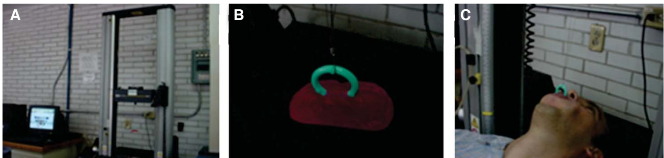
Figure 4. In vivo stress test. A) Universal testing machine. B) Buccal shield. C) Stress test.
