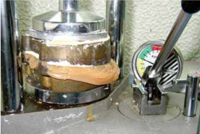
Figure 28. Muffle pressing with hydraulic press.
